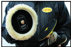
Attach a G Mop Twisted Wool Pad* to a polisher GMW801 (single sided) GMW806 (double sided)
