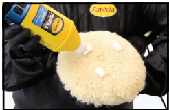
Spur new pads. Prime new pads with product. Apply a small amount of product to the surface or pad.
