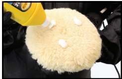
Spur new pads. Prime new pads with product. Apply a small amount of product to the surface or pad.
